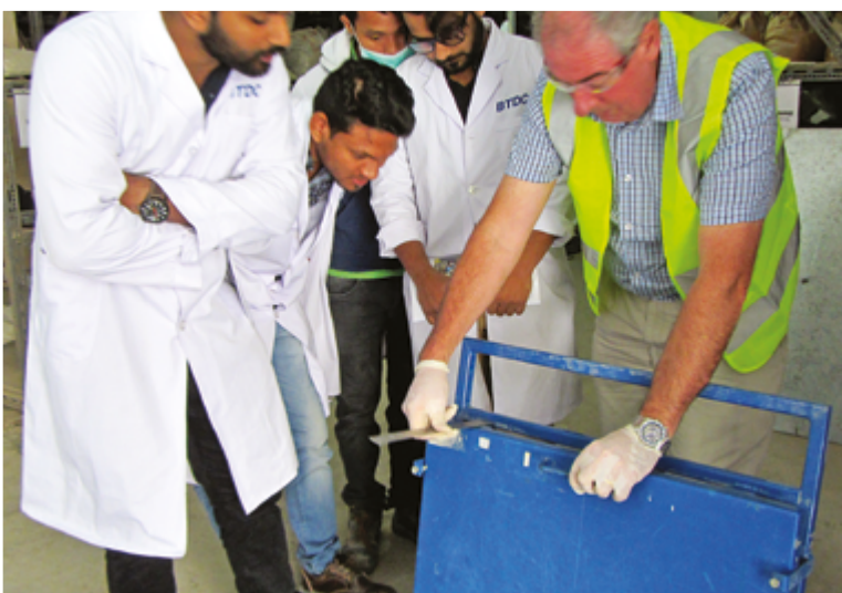
Checking flow table drop height before commencing test.
