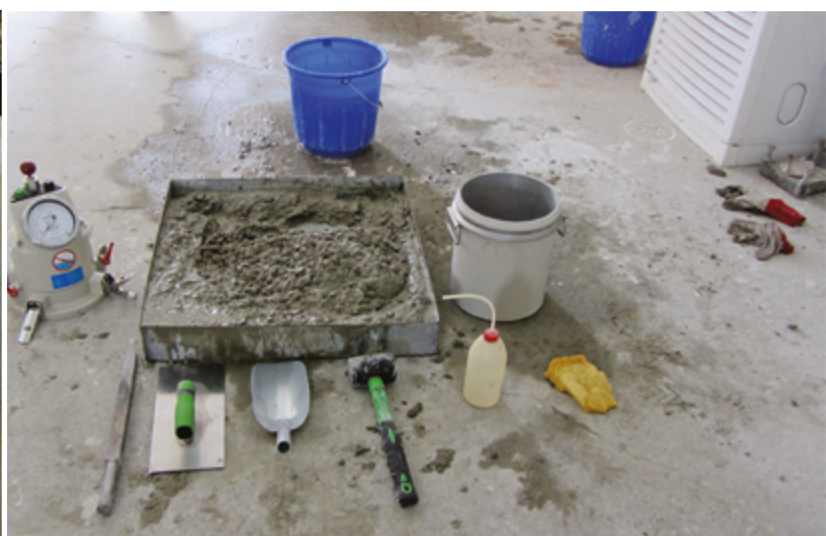
Air content test equipment set-up.
